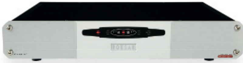
ABOVE: Caspian casework can house a choice of Roksan's PSUs and phono stages all within the same box. Front LEDs indicate what's under the lid
