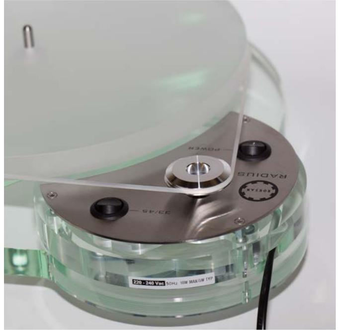
Remove the drive belt and gently place it around the platter and then onto the pulley. It is important to check that your mains supply frequency corresponds to the frequency specified on the Radius 7 mains input label.
